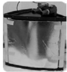
The soaking phase during the two different car usages imply the best thermal efficiency and thermal insulation to get the bigger calories amount available after 12h of parking. Fig. 2 Demonstrator of VIP integrated LTES for car and warm-up application
