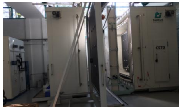
Fig. 3 Measurement of thermal bridge of panel VIP using hot box according EN ISO 8990
