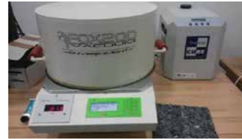
Fig. 1 Photo of device FOX 200 Vacuum from company TA Instruments during vacuum process
