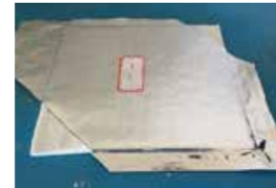
Fig. 1 VIP with the composite core material of aerogel-glass fiber mat produced by sol-gel method
