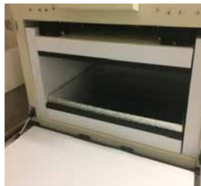
Fig. 1 Picture of vacuum insulation panel (VIP) sample in heat flowmeter to measure thermal conductivity
