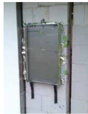
Fig. 2 STI demonstrator with dimensions 80 cm x 50 cm, installed at a massive test façade before surrounding insulating and plastering
