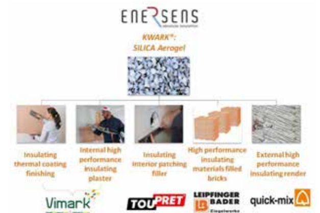
Fig. 1 Schema of the 5 insulation products developed within the Wall-ACE project
