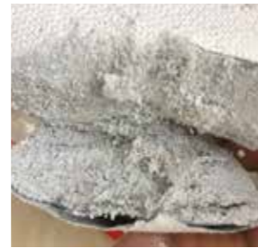
Fig. 2 Picture of a Hybrid Core Material composed of fumed silica, fly ash and glass fibers
