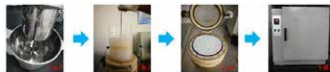
Fig. 1 Preparation process of the GWFs by wet process: (a) Beating; (b) Dewatering; (c) Forming; (d) Drying.
