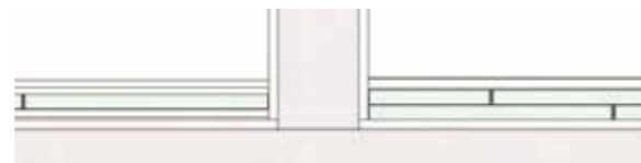
Fig. 5 Details of the model for hygro-thermal simulations considering single VIP's (core, envelope and air gap)
